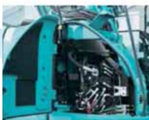
N&B (HAMMER/ZANGE) Ventil (optional) Multi-Steuerblock (optional)
