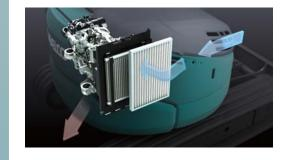
The high-density iNDr filter located at the mouth of the air intake duct helps prevent clogging of the cooling unit and air cleaner, thereby maintaining optimum performance. The corrugated filter cleans air through the tops of the ripples and collects dust at the bottoms of the corrugations to reduce clogging.
